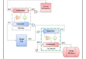
**Figure 2.** - This diagram depicts a typical interface of a Co-Therm machine with an existing chiller. The Co-Therm Fluid Heater developed and manufactured by TECSIR of Mexico is a machine using either HCFC22 or HFC134a that maintains 60°C water in the hotel water tanks. This machine replaces the duty of boilers and gas water heaters. The 2006-2008 market test in Puerto Vallarta Mexico had the machines installed in eight hotels using HFC 134a.
